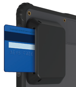
CAC Card Reader Module Available as an ODM option via rear chassis pogo-pin expansion slot
